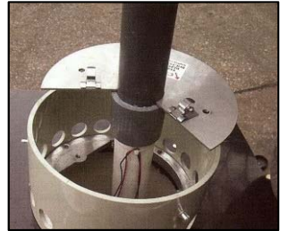
Pull up inner piping
