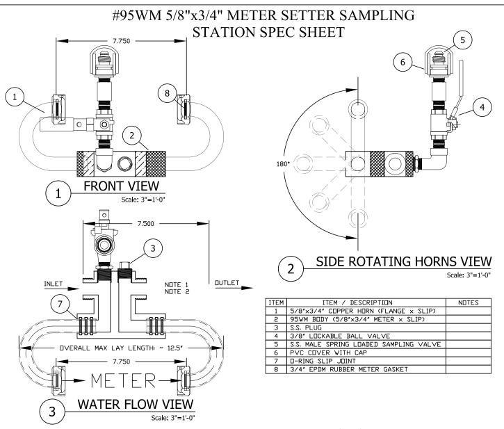
METER SETTER SAMPLING STATION SHALL BE METER BOX RETROFIT STYLE FOR A 5/8" x 3/4" METER, WITH 1" MIP METER THREADED INLET AND OUTLET, BOTH WITH A FACE FOR GASKET SEAL. IF DESIRED A DUAL CHECK VALVE (EITHER NYLON OR BRASS BODY) SHALL BE LOCATED BETWEEEN THE WATER METER AND RESIDENCE.
