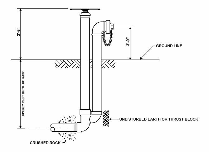
POST HYDRANTS SHALL BE NON-FREEZING, SELF DRAINING TYPE WITH A DEPTH OF BURY OF \_\_\_\_\_\_. THESE HYDRANTS WILL BE FURNISHED WITH A 2"FIP INLET AND A 2-1/2" NST OUTLET OR SMALLER. HYDRANT SHALL HAVE A NON-TURNING OPERATING ROD AND SHALL OPEN TO THE LEFT. ALL WORKING PARTS SHALL BE BRONZE TO BRONZE DESIGN AND BE SERVICEABLE FROM ABOVE GRADE WITH NO DIGGING. HYDRANTS SHALL BE MANUFACTURED BY KUPFERLE FOUNDRY CO., ST. LOUIS, MO, OR APPROVED EQUAL.
