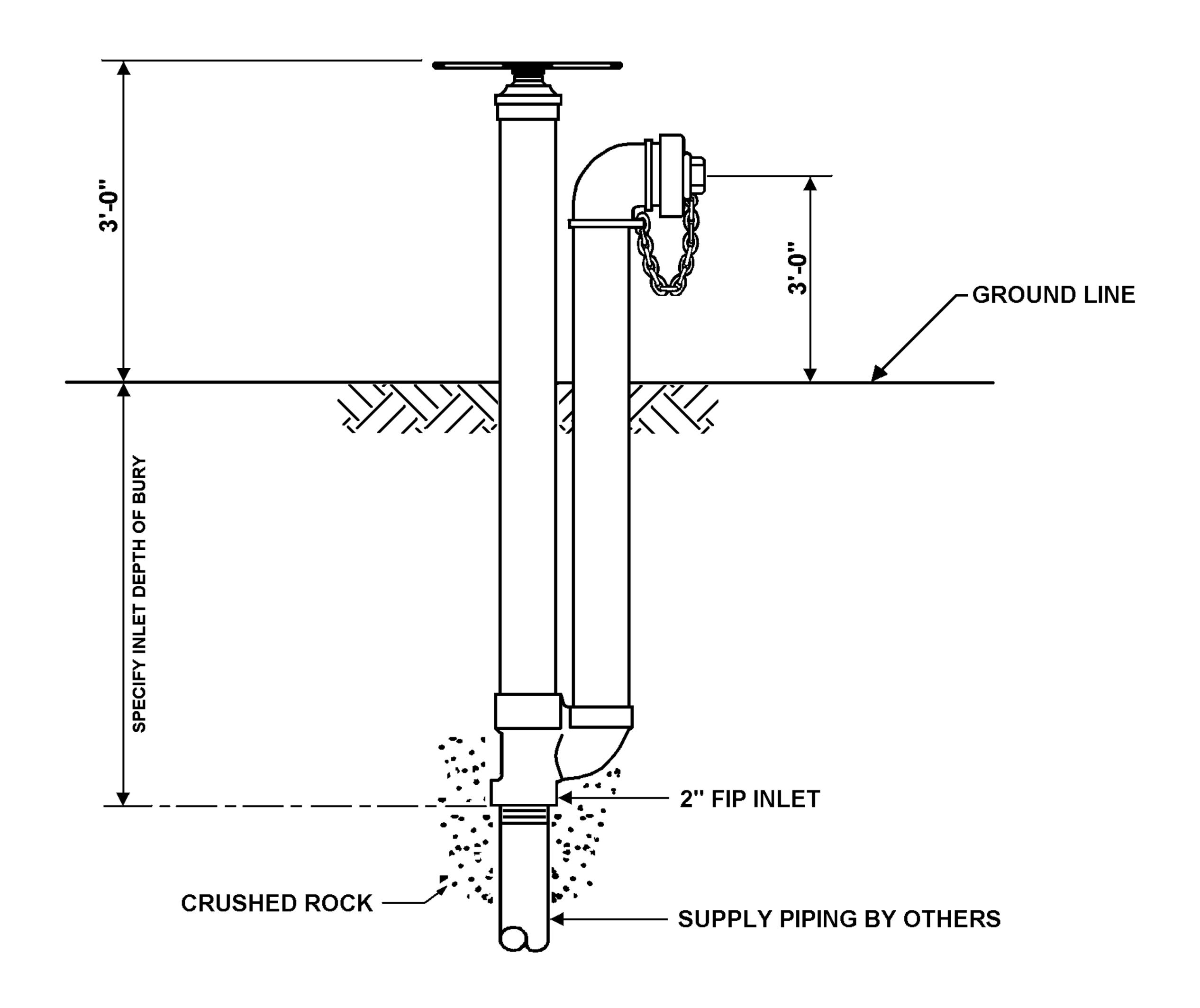
POST HYDRANTS SHALL BE NON-FREEZING, SELF DRAINING TYPE WITH A DEPTH OF BURY OF \_\_\_\_\_\_. THESE HYDRANTS WILL BE FURNISHED WITH A 2' FIP INLET AND A 2-1/2" NST OUTLET OR SMALLER. HYDRANT SHALL HAVE A NON-TURNING OPERATING ROD AND SHALL OPEN TO THE LEFT. ALL WORKING PARTS SHALL BE BRONZE TO BRONZE DESIGN AND BE SERVICEABLE FROM ABOVE GRADE WITH NO DIGGING. HYDRANTS SHALL BE MANUFACTURED BY KUPFERLE FOUNDRY CO., ST. LOUIS, MO, OR APPROVED EQUAL.
