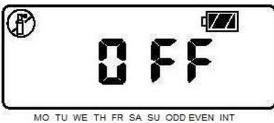
9. 'Manual/test flush' (this screen will only appear after right arrow is held down)
