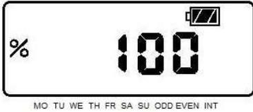
The controller will default to 100% and can be adjusted by using the  $\oplus$  or  $\ominus$  buttons. This field will adjust in 10% increments. The percentage shown on this page will impact the **duration** of the programmed flushes. For example, if you have 20 minute flushes programmed, and you adjust this field to 50%, the programmed flushes will run for 10 minutes.
