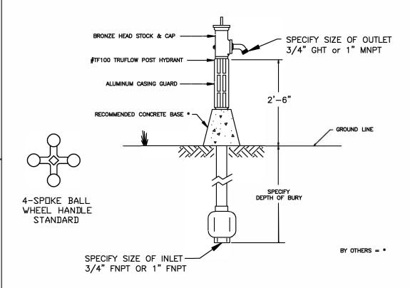
Hydrant shall be  $\_\_$  ' Depth of Bury with a 3/4" or 1" FNPT vertical inlet and a 3/4" GHT or 1" MNPT outlet.
