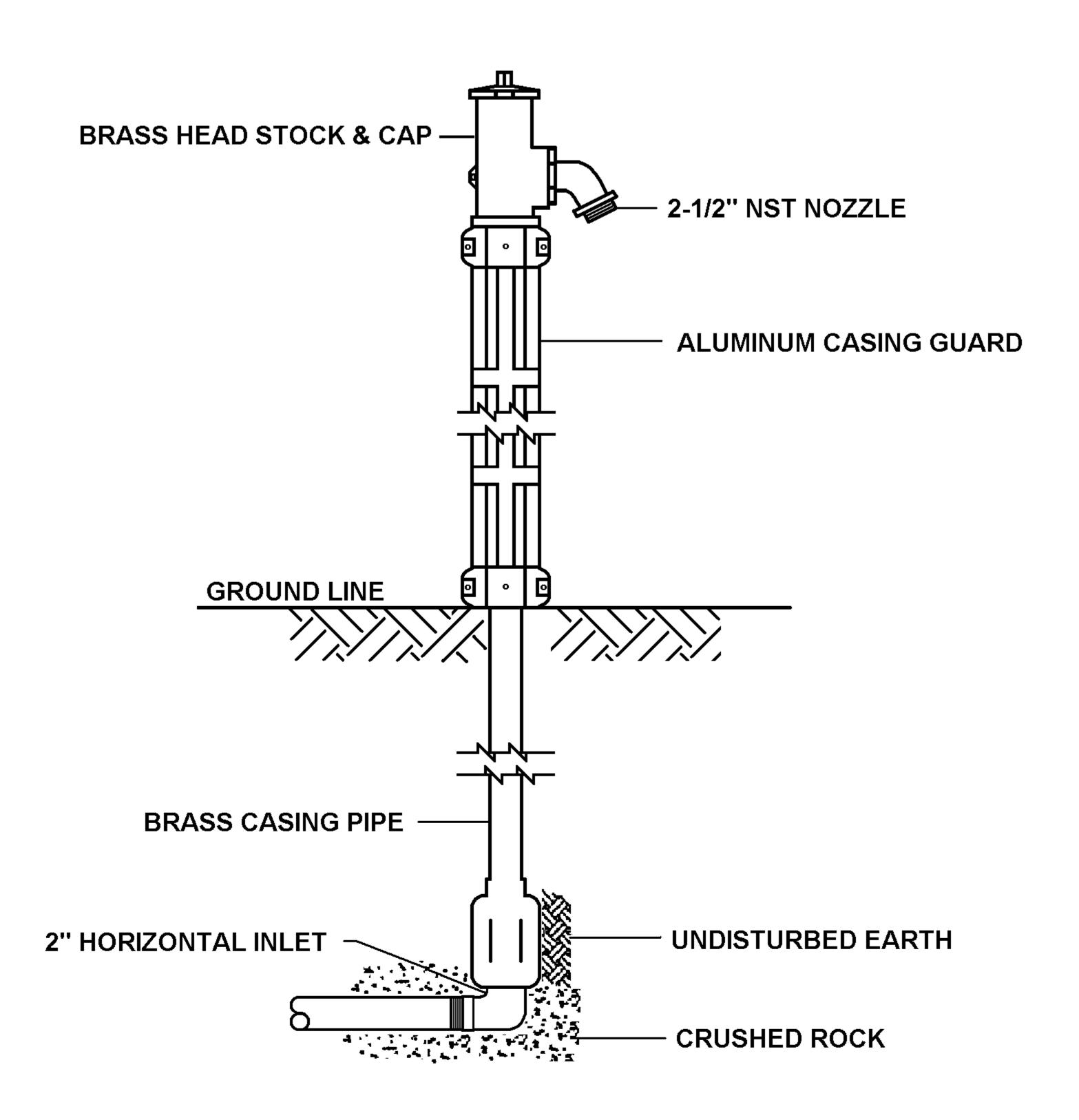
POST HYDRANTS SHALL BE NON-FREEZING. SELF DRAINING TYPE WITH A \_\_\_\_\_\_ DEPTH OF BURY. THESE HYDRANTS WILL BE FURNISHED WITH A 2" FIP INLET, A NON-TURNING BRASS OPERATING ROD AND BRASS CASING PIPE. HYDRANT SHALL OPEN TO THE LEFT. ALL WORKING PARTS SHALL BE BRONZE TO BRONZE DESIGN AND SERVICEABLE FROM ABOVE GRADE WITH NO DIGGING. THE OUTLET SHALL ALSO BE BRONZE WITH A 2-1/2" NST NOZZLE OR SMALLER. HYDRANTS SHALL BE MANUFACTURED BY KUPFERLE FOUNDRY CO., ST. LOUIS, MO. OR APPROVED EQUAL.
